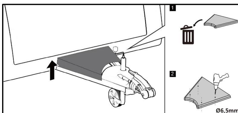
Remove the A-frame cover from the A-frame (1) or drill holes in the A-frame cover for the U-bolts (2).
