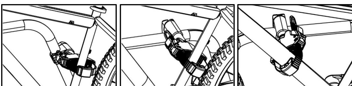
Front wheel straps to secure the front wheels against turning.
