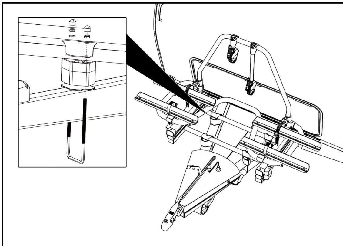
To make sure that the carrier remains in its position, it must be secured with the four screws. To do so, 4 small holes (4 mm) must be drilled in the base part, after which the clamp and the base frame can be screwed together.
