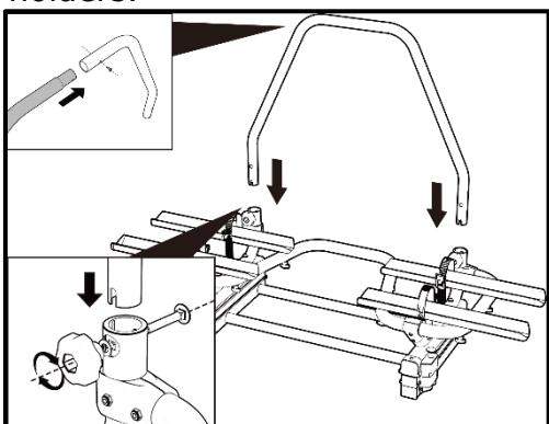
Secure this U-tube with the supplied carriage bolts (M8x60), washers and plastic rotary knobs. Make sure the plastic rotary knobs are on the frontside (see drawing).
